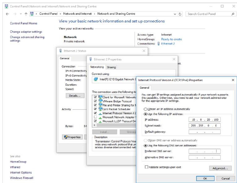
Figure 2: Setting the IP address manually in Windows
