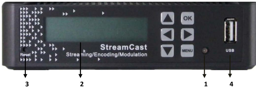
1. **Power status indicator:** This LED light is turned on when the StreamCast is power on.
