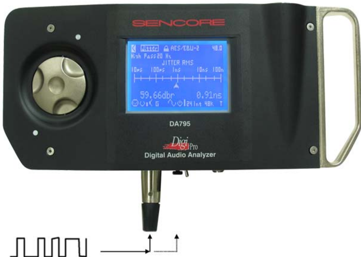
Figure 4. Jitter measurement of an AES Digital Audio Input taken with a Sencore DA795 Digital Audio Analyzer.
