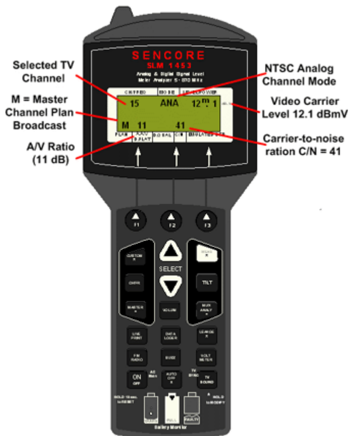
Figure 4 – The Sencore SLM1453 measures and displays the video level dBmV, A/V ratio dB and C/N ratio dB of an analog NTSC TV signal.
