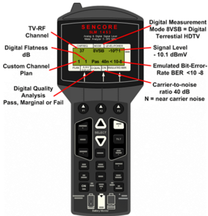
Figure 9 – The SLM1453 measures the digital TV signal level, flatness, C/N ratio, Bit-error-rate BER and provides a total quality analysis indicating pass, marginal or fail.
