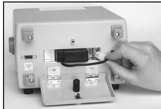
Fig. 6: The optional BY289 is installed in the LC103 for portable operation.
