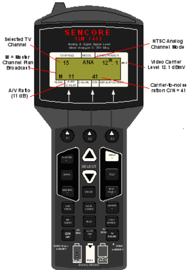
Figure 4. NTSC analog signals should be tested for video carrier level, A/V ratio, and C/N ratio.
