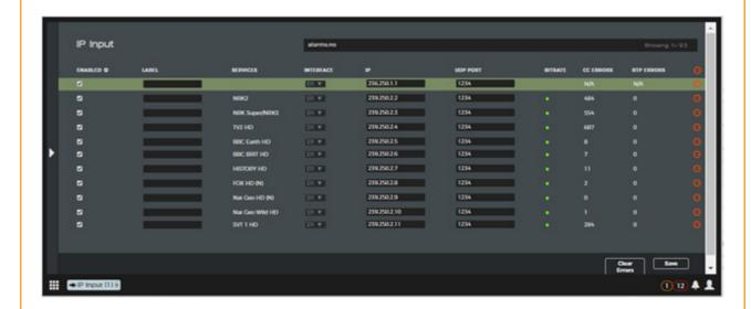
The new source appears in the input list view, highlighted. It is now possible to make changes before saving the changes to the system. Once saved the input analysis starts and indicates if the input is available via the bitrate, CC counter and the RTP counter. If the input contains DVB services they will be listed under services column.
