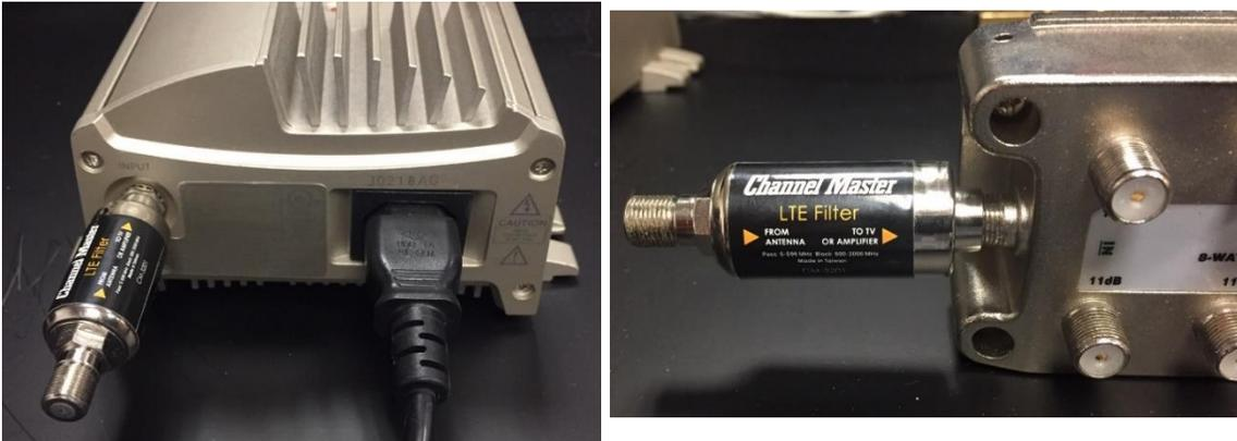
For Sencore AtlasGear frames with AG2600/4400/5800/6000 receiver cards, the RF input port is a BNC connector. The Sencore kit includes a short BNC cable as an option for installing LTE filter(s) as shown below. Connect the cable from the output side of the LTE filter to the cable and the other end of the cable to the RF input port as shown.
