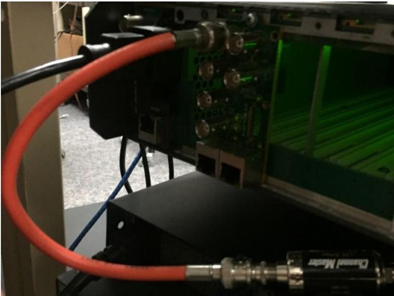
For Sencore MRD receiver/decoders/gateway products with an 8VSB receive card or capabilities, locate the RF input to the receiver. These products use a traditional F-connector. The LTE filter output side may be connected directly to the input F connector as shown below. Connect the signal input from the antenna to the input side of the LTE filter.
