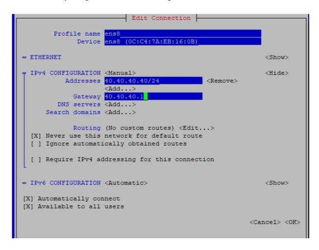
Selecting **Automatically connect** will ensure the interface is connected next time the system boots.
