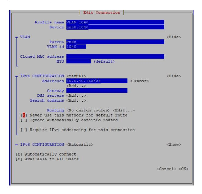
After entering the configuration for the VLAN interface select **OK** to return the previous menu, then select **Back** and finally **Activate a connection** to activate the newly created VLAN interface.
