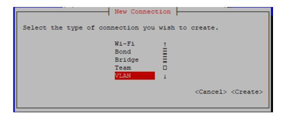
Edit the settings for the VLAN interface. The Device field should contain the name of the physical interface to be used for this VLAN and the VLAN number, for example ens8.1040 means VLAN 1040 on interface ens8. The parent and VLAN ID fields should correspond to the values in the name field. In our example ens8 is the parent and 1040 is the VLAN. Other settings are the same as for normal IPv4/6 interfaces.
