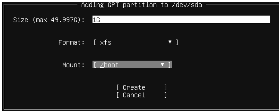
Figure 1.5: Create boot partition
