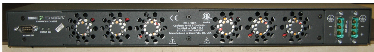
Figure 4.2: VB300-DC rear: two –48V DC connectors located on the the right
