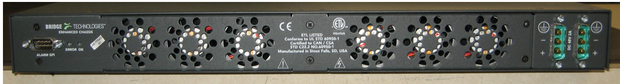
Figure 4.2: VB300-DC rear: two –48V DC connectors located on the the right
