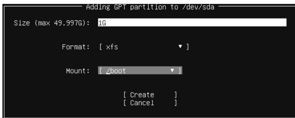
Figure 3.5: Create boot partition
